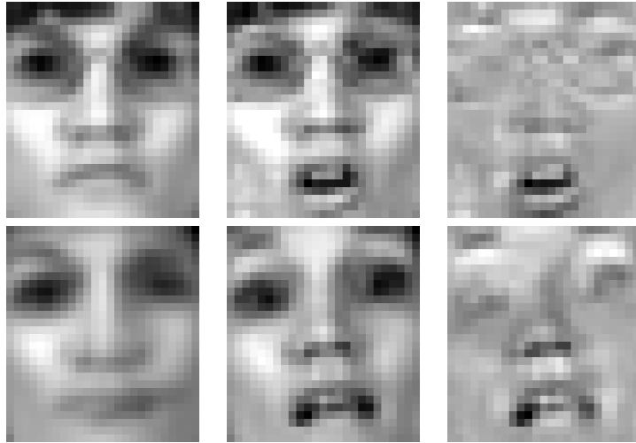
Figure 5.6. Examples of two mean face difference images. From left to right: Mean face, face patch, mean face difference image
