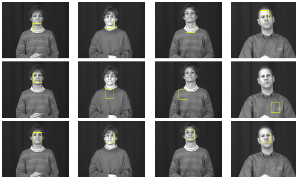
Figure 7.9. Sample frames of experiments with different score functions for head tracking in different videos. The following score functions are used (from top to bottom): brightness, eigenface, combination of brightness and eigenface.
