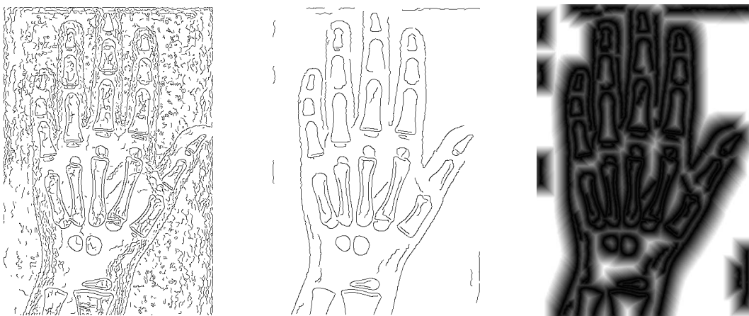
Figure 5. Left: binary contour image of a hand radiography. Middle: binary contour image after removing irrelevant contours. Right: distance transformed contour image (contrasted due to visualization aspects).
