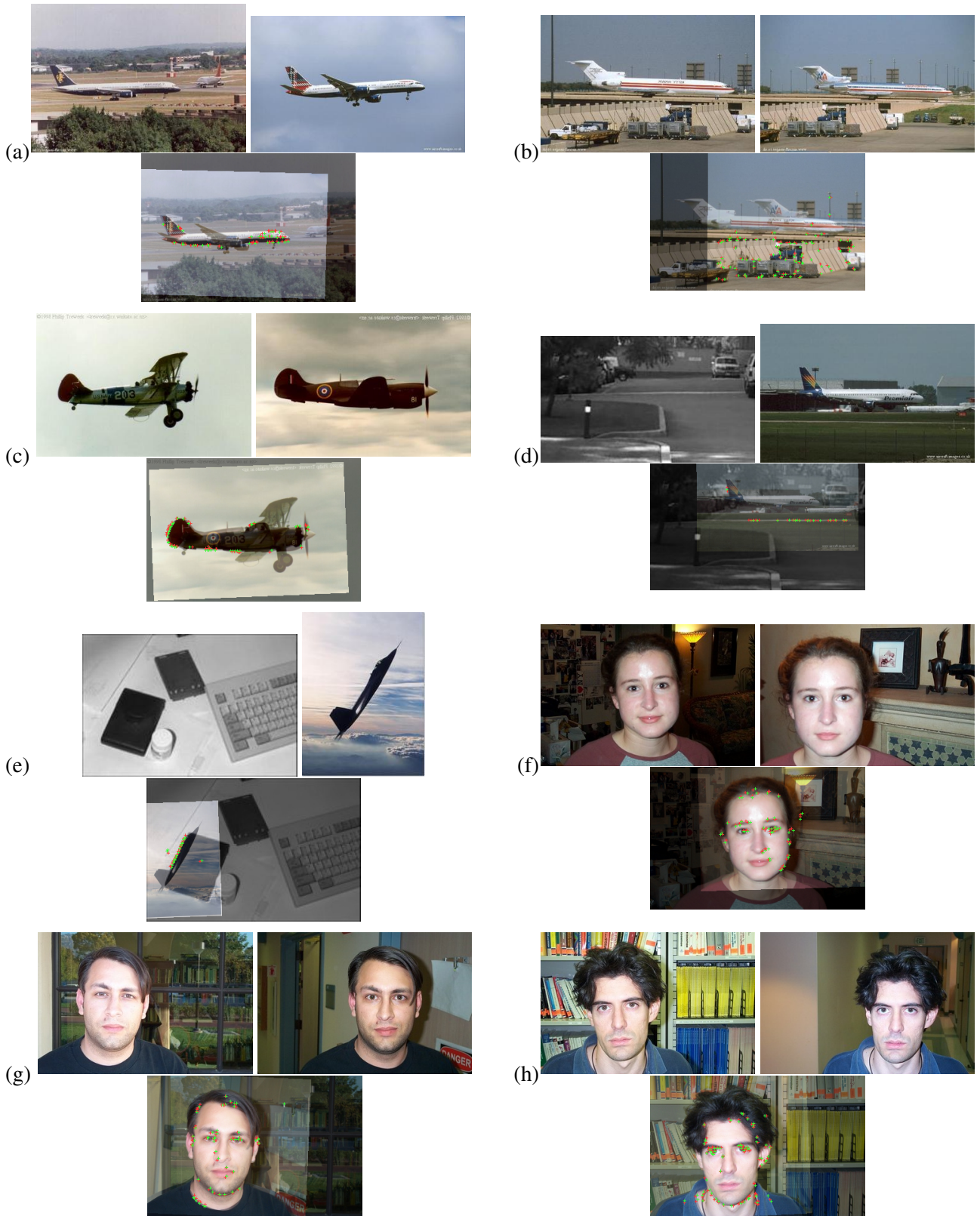
Figure 4: Examples of matching results. Each triple of images shows (top row) the test image, the matched reference image, and the reference overlaid on the test image after application of the determined transformation (bottom row). The crosses show the position of the matched patches. Note that we only match to reference images showing an object of the category and decide about presence or not using the average matching scores.
